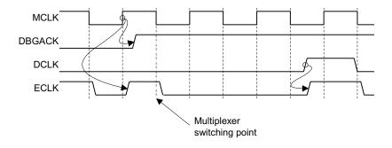
Figure 5-4 Clock switching on entry to debug state
