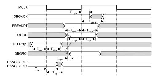
Figure 7-13 Debug timing
