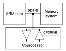
Figure 4-5 Coprocessor connections with bidirectional bus
