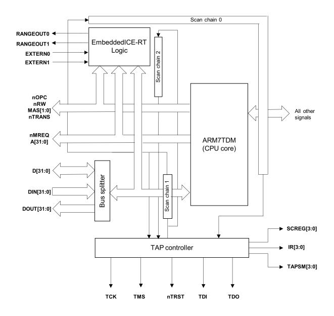
Figure 1-2 ARM7TDMI processor block diagram
