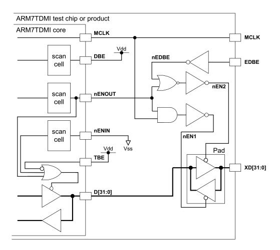
Figure 3-17 Test chip data bus circuit
