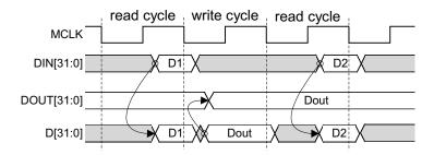
Figure 3-13 Unidirectional bus timing
