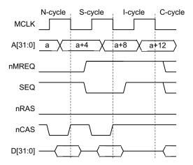
Figure 3-4 Internal cycles
