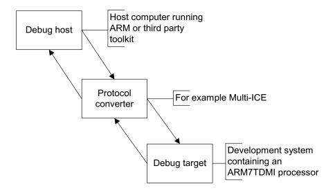
Figure 5-1 Typical debug system
