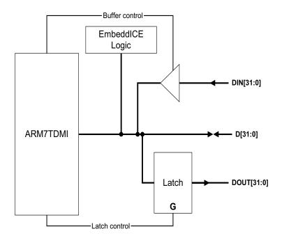
Figure 3-11 External bus arrangement
