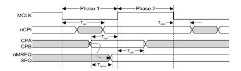
Figure 7-10 Coprocessor timing
