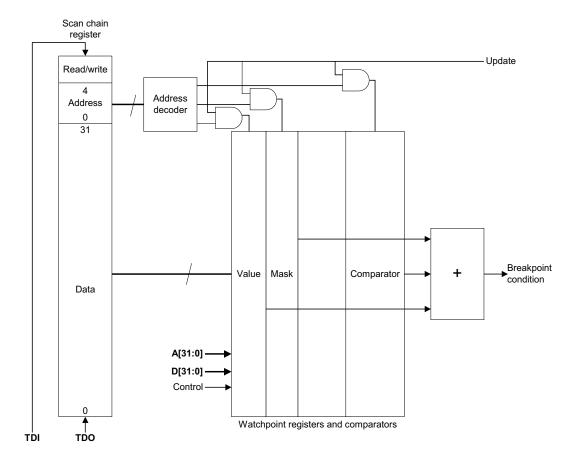
Figure B-7 EmbeddedICE-RT block diagram
