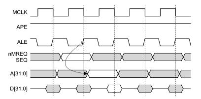
Figure 3-10 SRAM compatible address timing
