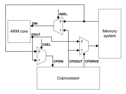
Figure 4-6 Coprocessor connections with unidirectional bus
