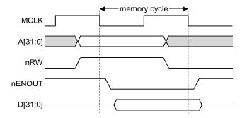
Figure 3-15 Data write bus cycle
