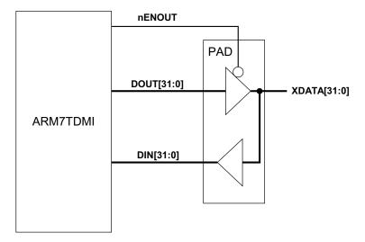
Figure 3-14 External connection of unidirectional buses
