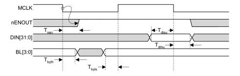
Figure 7-8 Unidirectional data read cycle
