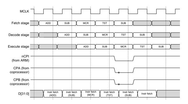
Figure 4-3 Coprocessor data operation sequence
