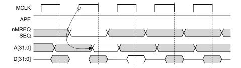
Figure 3-8 Pipelined addresses
