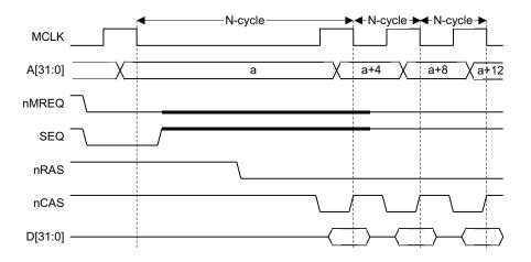
Figure 3-3 Sequential access cycles
