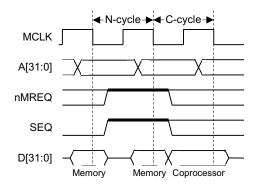
Figure 3-6 Coprocessor register transfer cycles
