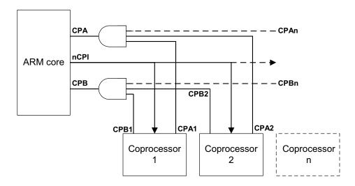
Figure 4-7 Connecting multiple coprocessors
