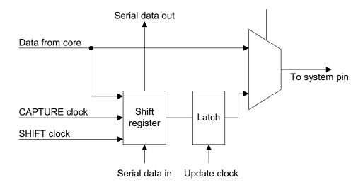
Figure B-4 Output scan cell
