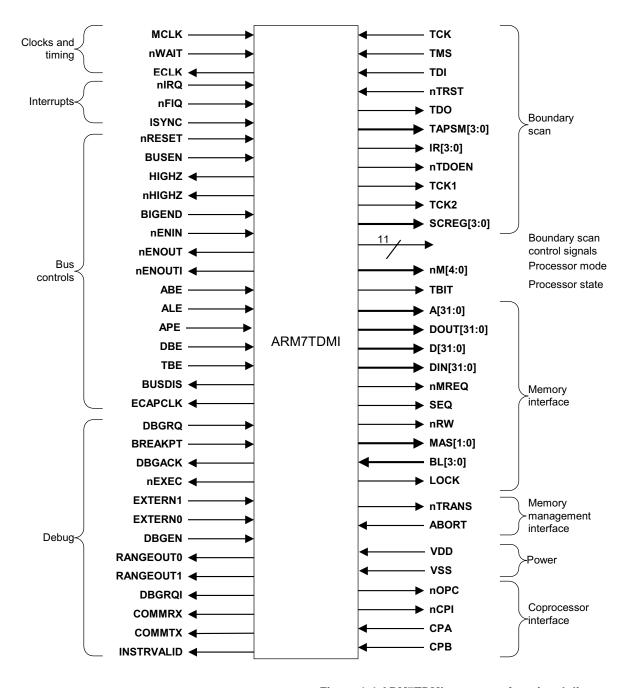
Figure 1-4 ARM7TDMI processor functional diagram
