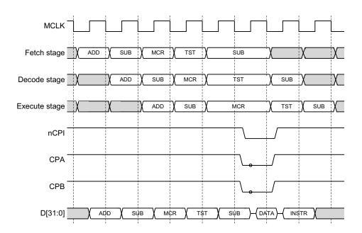
Figure 4-2 Coprocessor register transfer sequence
