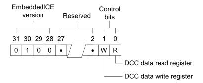
Figure 5-6 DCC control register format
