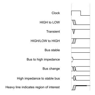
Figure Pre-1 Key to timing diagram conventions
