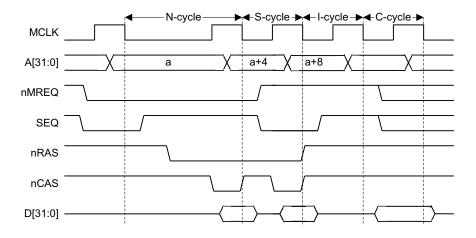
Figure 3-7 Memory cycle timing
