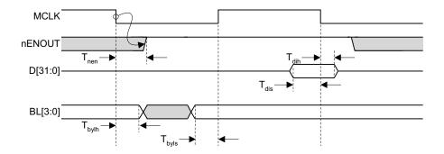
Figure 7-4 Bidirectional data read cycle
