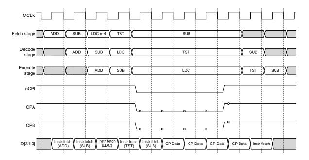
Figure 4-4 Coprocessor load sequence
