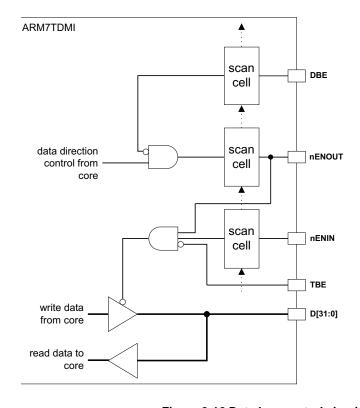
Figure 3-16 Data bus control circuit
