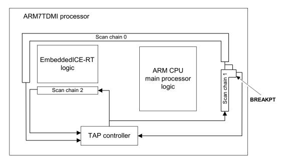
Figure 5-2 ARM7TDMI block diagram
