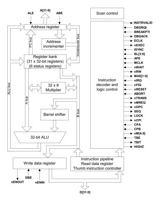
Figure 1-3 ARM7TDMI main processor logic
