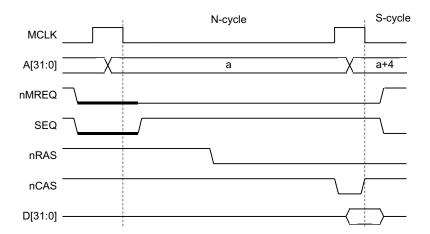
Figure 3-2 Nonsequential memory cycle
