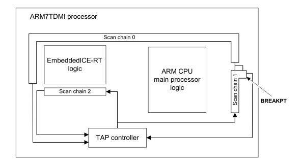
Figure B-1 ARM7TDMI core scan chain arrangements
