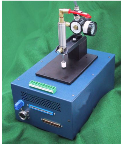
Figure 3-3: Theta JC Measurement Setup
