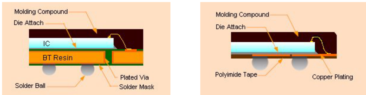
Figure 1-8: Rigid BT-based Substrate Chip Scale Packages, left; Flex-Based Tape Substrate, right
