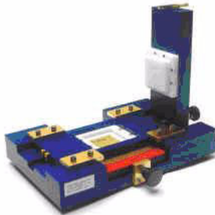
Figure 4-1: Altair BGA Fixture used for TDR measurement
