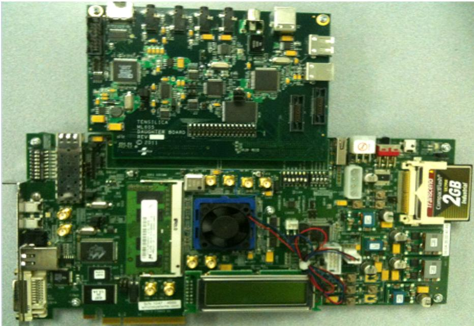
Figure 5–9. Connection of XT-ML605-D Daughter Board and XT-ML605 Board
