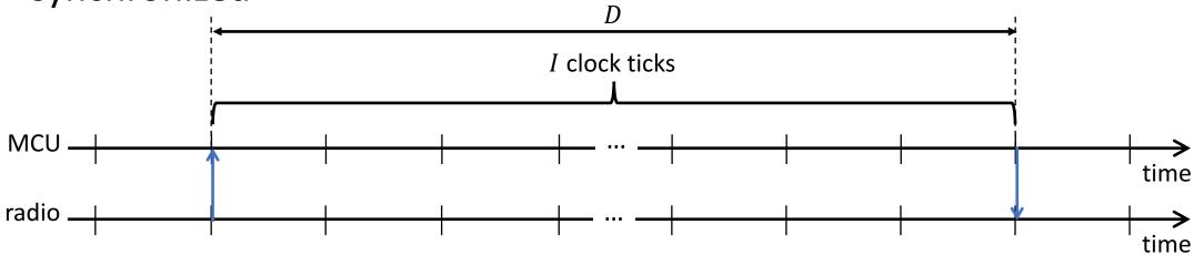
• So the delay is simply the time the MCU needs to execute for 100 clock ticks:  $D = \frac{I}{f} = \frac{100}{8000000} = 12.5 \mu \text{s}$
