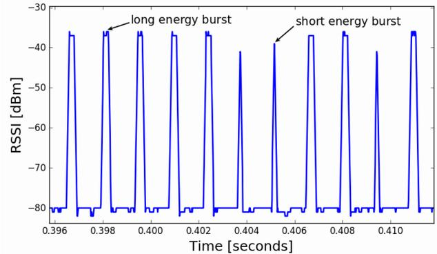
**Figure 3. Visualization of CTC energy pattern recorded by a TelosB.** Due to averaging effects, the short energy bursts seem to have a lower RSSI level than the long energy bursts, and appear as spikes rather than plateaus.
