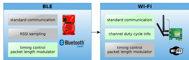
Figure 1. Illustration of our holistic CTC approach with the example of BLE to Wi-Fi communication
