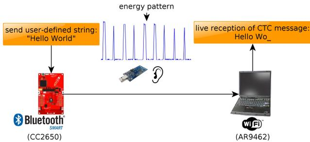
**Figure 2. Demonstration setup.** A BLE device transmits a user-defined string to a Wi-Fi device. The resulting energy patterns are observed with a passive TelosB sniffer.
