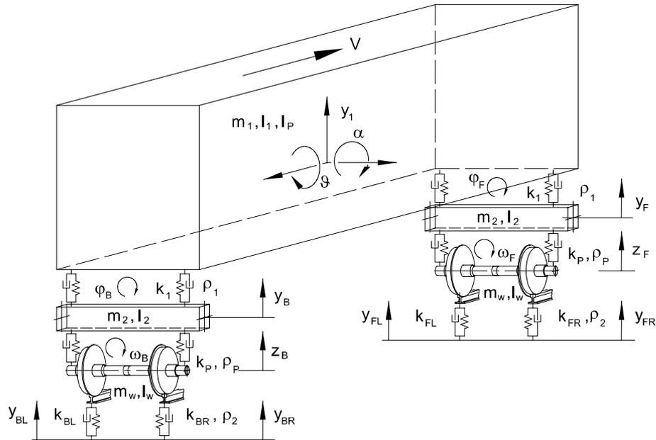
Figure 2. Multibody system: coach, bogie, wheelset, primary and secondary suspension and track.
