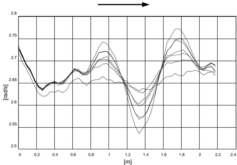
Figure 7. Measured angular velocity (pitch) of the coach under varying track conditions, journey there. The arrow indicates the direction of the train velocity along the track.
