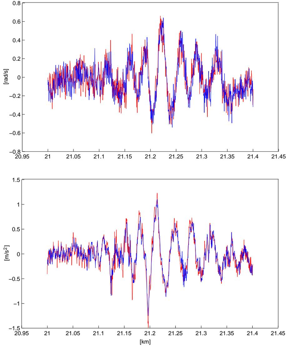
Figure 5. Above pitch angular velocity  $\dot{\alpha}$  and below vertical acceleration  $\ddot{y}_1$  of the coach response to the onset of a curve (at km 21.2).
