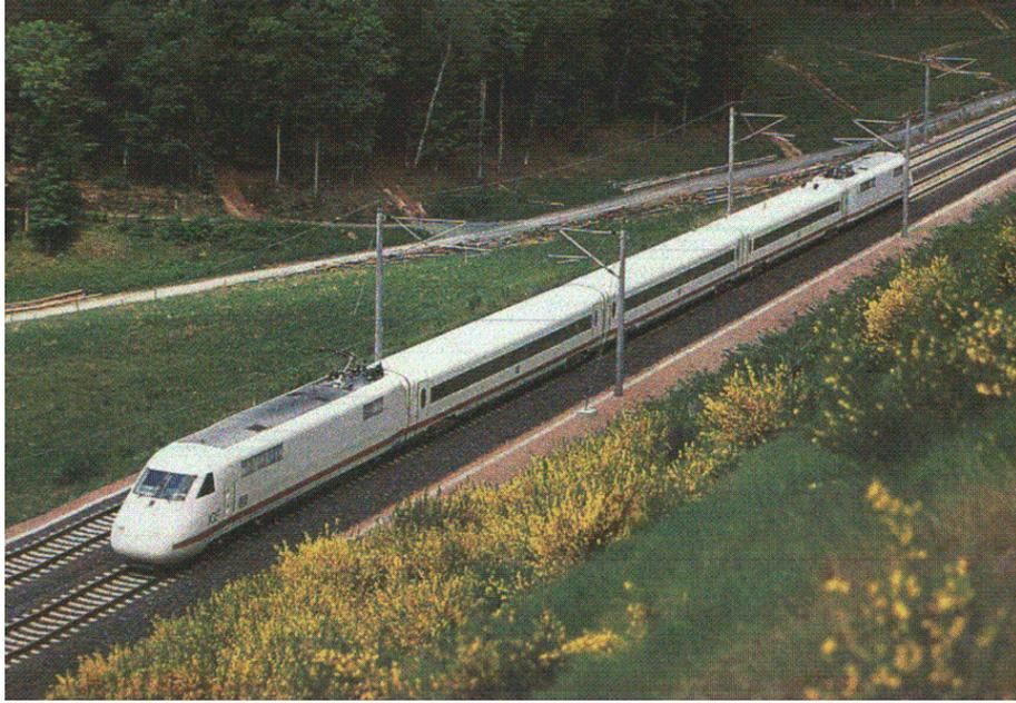
Figure 1. Special measurement train ICE-V, predecessor of ICE-S.
