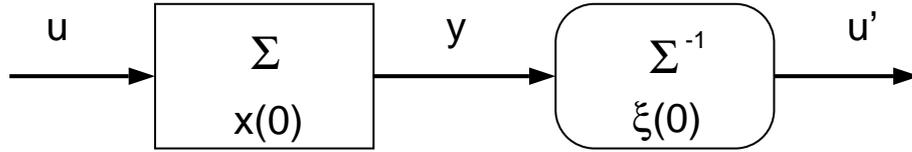
Figure 3. Inversion of a dynamic system: the output  $y$  of the system becomes the input of the inverse system.  $x(0), \xi(0)$  are the initial states of the system and its inverse.
