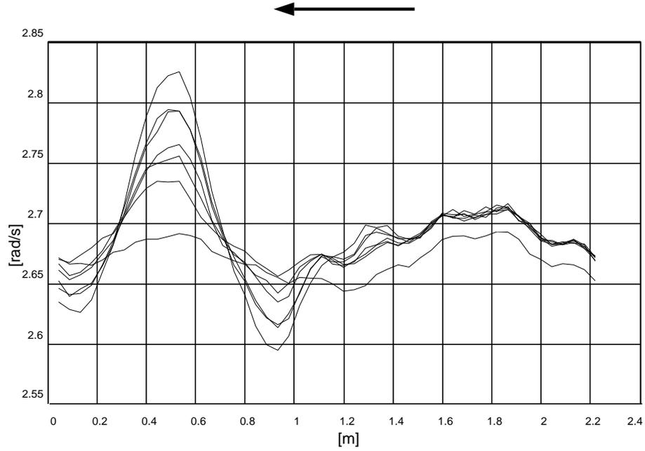
Figure 8. Measured angular velocity (pitch) of the coach under varying track conditions, return journey.
