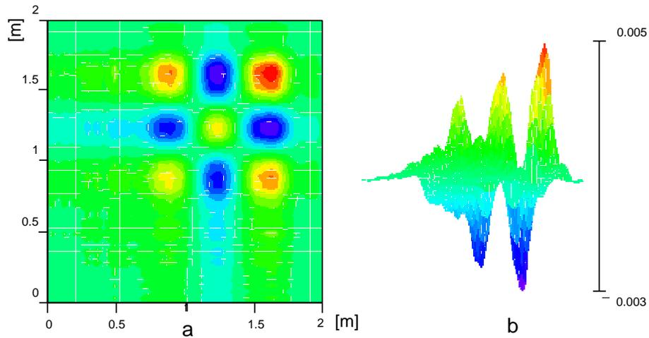
Figure 9. Covariance matrix  $\mathbf{C}_{uu}$ : a) contour-plot the  $x, y$ -axes represent the matrix indices corresponding to the piece of track, the value of the matrix entry is color-coded, b) perspective view on  $\mathbf{C}_{uu}$  onto its diagonal.
