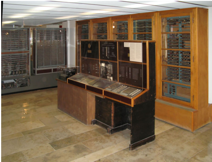
Zuse Z4 (1950) with Ferrit kernel storage and multiple punch card reader
