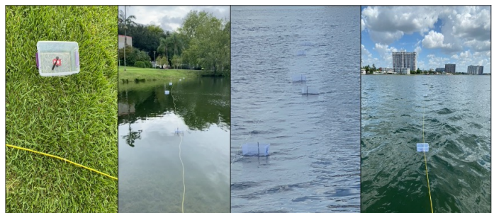
Fig. 2: A wireless sensor network consisting of nodes placed inside open floating boxes and deployed on the surface of different water bodies.
