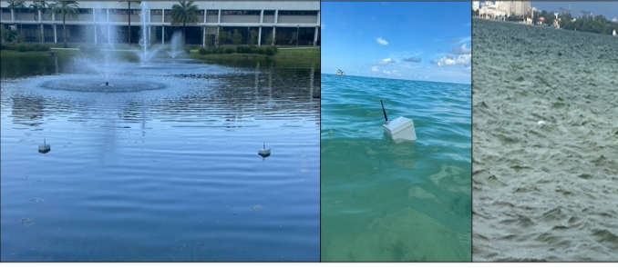
Fig. 3: A wireless sensor network (with nodes sealed in waterproof boxes) deployed on the surface of different water bodies.
