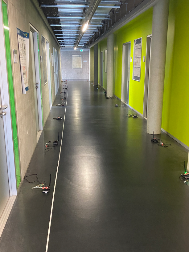
Fig. 3: Deployment of a wireless sensor network along a corridor.
