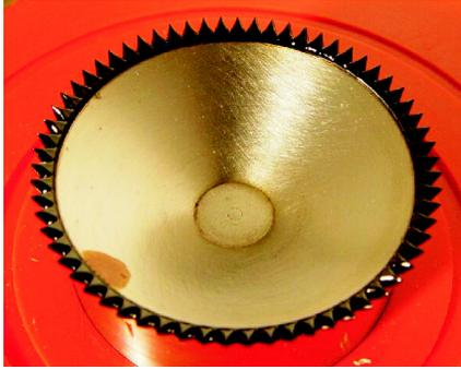
**Fig. 5.** The MF EMG 901 trapped by the gradient magnetic field at the sharp edge of a pole shoe of an electro magnet. The diameter of the pole shoe is 40 mm
