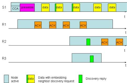
Fig. 6. Handover mechanism in MA-MAC
