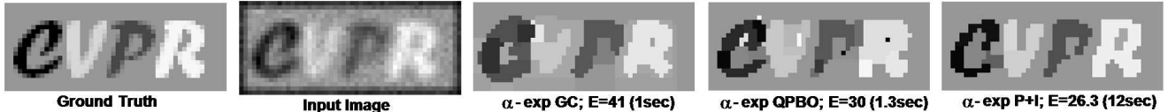
Figure 3. Image deconvolution. Given a blurry and noisy input image with 32 gray-levels, the task is to reconstruct the ground truth. The new P+I method within alpha-expansion improves results compared to graph cut and QPBO-based alpha expansion both in terms of energy and visually. Note, for all alpha expansion based methods the order is crucial. Energies of P+I differed between 26.3 and 27.9 and runtime between 12 and 31 sec, best result shown. Also, to improve runtime of P+I we initialized it with standard graph cut based alpha expansion. BP (E=103), TRW (E=112) and ICM (E=54) perform poorly. Simulated annealing achieved a similar result to P+I in 60 sec.
