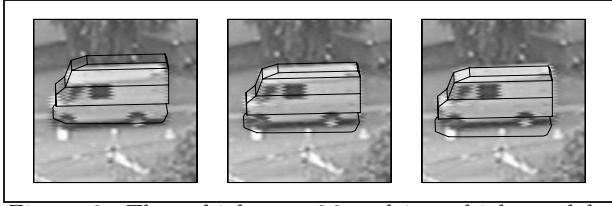
Figure 2: The vehicle no. 26 and its vehicle-model, which was initialised in half-frame 2140 of the image sequence "stau03". The result with the old method and without interactive adjustment is shown in the left image. The middle image depicts the result with the old method and with interactive adjustment. The right image shows the result with the new automatic method.
