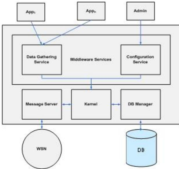
Fig. 1. The conceptual architecture of the Senceive Middleware
